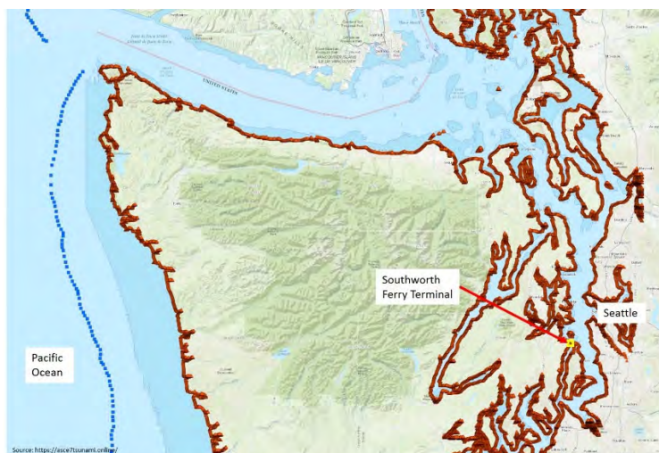
Snapshot from ASCE Tsunami Design Geodatabase. Blue dots indicate offshore tsunami amplitude data points, orange dots indicate runup elevation data points.
