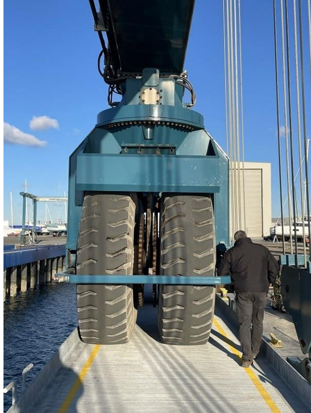
6 - Wheels of the movable Marine Travellift
