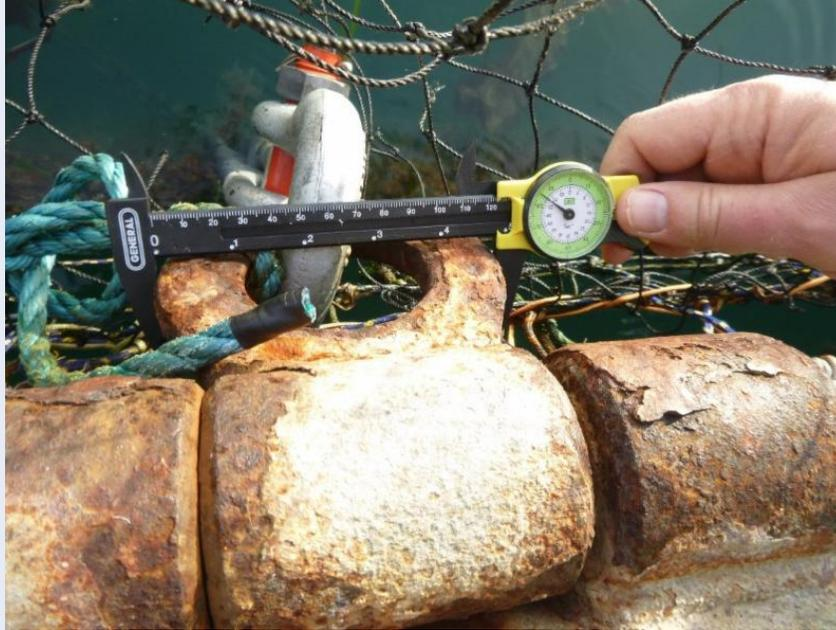
*Corrosion may have been a factor in the failure of the net pen at Cypress Island.*
